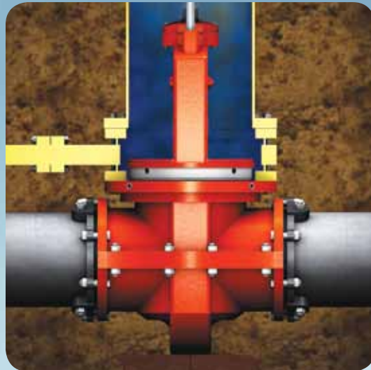
Step 2 Insert bonnet into the valve body.
