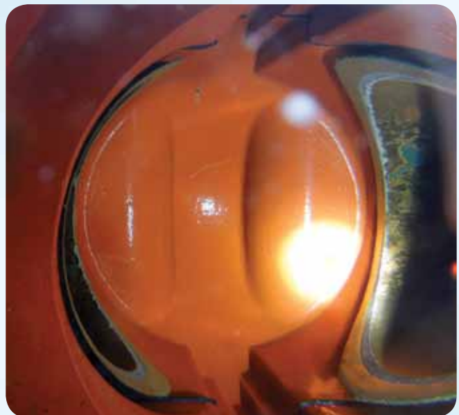
An under-pressure look of clean valve seat.
